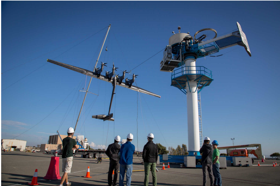
Figure 1: 600 kW “drag power” prototype of Makani Power/Google (image source: https://www.solveforx.com/media/story/makani/hero.jpg , accessed: March 7, 2016).
